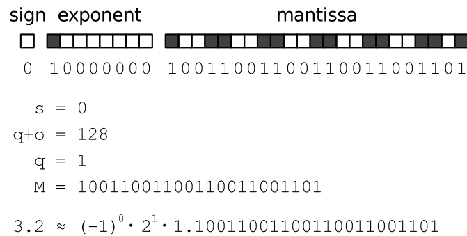
Figure 3: Representation of 3.2 in binary32 format
